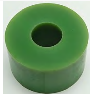
Roller Green Polytube, 3-5/8" OD X 1-3/8" ID X 2" LG, 60 Duro
