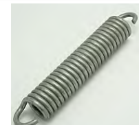
Spring, 1-5/16" OD X 13/16" ID X 8" Long, .225 Wire, With Hooked Ends
