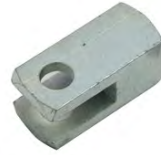
Clevis, 240, 310, 050, Hardware, 1/2-20 National Fine Thread 1.69 Long .38 Pin, Bimba Cylinder Bracket
