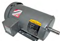
Motor, 3-HP, 3450 RPM, 145T Frame, 208/230-460V, 60 Hz (979, DL-2)
