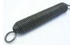
Spring 1.75 OD 14 Long Swivel Enclosed Hook Both Ends 207 Wire Dia. (990 F4 Front Section, Vertical)
