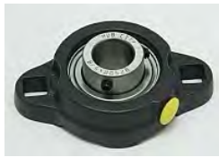
Bearing, FB 160 X 5/8", 2 Square Hole Mount, Setscrew Locking Relube
