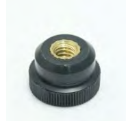
Knob, DK-42, Knurled, 3/4 Dia. 1/4-20 Female Insert 5/16 Thread Depth.
