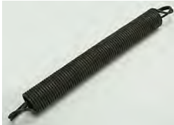
Spring, 1-5/16" OD X 1" ID X 12" Long, .135 Wire, With Hooked Ends
