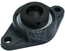
Bearing, FB 230 X 1-1/4", 2 Hole Mount, Eccentric Locking Collar Relube.
