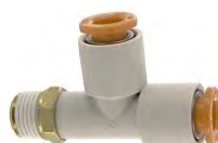
Fittings, SMC, Male Run Tee KQ2Y Series, 1/4 Tube OD X 1/4 NPT
