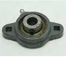
Bearing, FB 160 X 1/2", 2 Square Hole Mount, Setscrew Locking Relube
