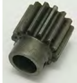
Spur Gear, YSS 1614 X 1/2, With Relief Machined on the Gear End, Modified Bore Hardened & Honed, 5/32 Roll Pin, OAL 1.170
