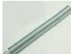
Spring, 1-1/16" OD, 12" Long, .135 Wire, 10.5" Stretch 7.775 Lbs/Inch, 18 Initial Tension
