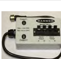
BANNER PORTABLE DEMO BOX SENSOR TESTER KVAL P/N: DBQ5
