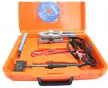
UT-236 Weld-Splice Kit for V-Belt Splicing
