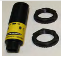
S182VNFF100Q8 Diffuse Photo Eye 24 Volts DC 3.9" Fixed Field 18MM Dia. NPN (Banner) (Uses M12 4 Pin Cord Not Included) Substitute for: DIFUSEFF4-M12-BLK KVAL P/N: BANS182VNFF100Q8
