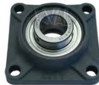
Bearing, FB 250 X 1-1/4", 4 Hole Mount, Setscrew Locking Relube.
