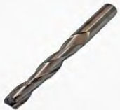
Router Bit, Solid Carbide, 7/8" Dia. X 7/8" Shank X 8" OAL X 2.2" CL Up Cut, 2 Flute Rougher With 5-1/2" Spiral Relief
