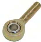
Rod End Male, TRE-6, 3/8 Bore, 3/8-24 Male Thread Shank End
