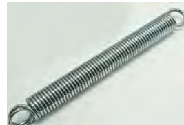
Spring, 1-1/4" OD X 7/8" ID X 12" Long, .162 Wire, Double Loop Each End
