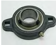
Bearing, FB 160 X 1-1/4", Short Base, 2 Square Hole Mount, Setscrew Locking Relube.
