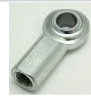
Rod End Female, TRE-12, 3/4 Bore, 3/4-16 Thread Shank End
