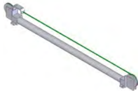
Cylinder, Cable Greenco Cable-Trol, CD2047, Used on Handler Carriage
