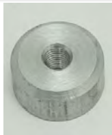
Pad, Aluminum, 1" Dia., 3/8" Thick, 5/16 NF Thread
