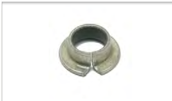
Flanged Garlock Bushing, 3/8" I.D. - .4684 O.D. X 1/4" Long
