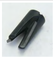
Router Bit, Spin On, 1/2" +.005" Dia., 1/4-28 Thread, Reverse Helix.
