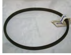
V-Belt, B34, 37 Outside Length, 35.8 Pitch, 5L370
