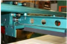
Foam, Grabber, Foam Pad for Resting Beams, 1" Thick X 2-1/4" Wide X 35" Long
