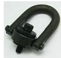
Hoist Ring, 2500 lbs Capacity, 360 Deg. Swivel, 180 Deg. Pivot
