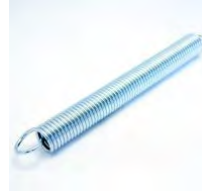
Spring 1-3/16-OD X 7/8-ID X 12 Long, .162 Wire Hooked Ends
