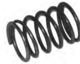
Spring 19/32-ID X 1-1/16 Long, .062 Wire 6 Coils Ground Ends
