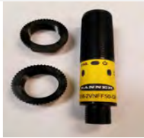
S182VNFF50Q8 24 Volts DC 2" Fixed Field 18MM Dia. NPN (Banner) (use M12 4Pin Cord) Substitute for DIFUSEFF2-M12 KVAL P/N: BANS182VNFF50Q8
