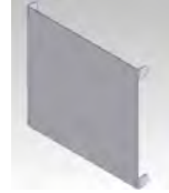
CAGE LABEL PLATE, ELECTRO GALVANNEALED STEEL 24 GA X 5-3/4 X 6.189 WITH TABS AT CORNERS.
