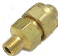
Air Nozzle, UniJet Blow-off nozzle, 1/8 Male Thread, .023in Slot Width
