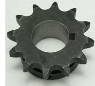
Sprocket, 50B12, Modified Bored to 1-1/8" With 1/4 Keyway and 1/4 -20 SS at 0 and 90 Deg.
