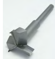
Router Bit, 3-Wing, 2-3/8" Dia., Carbide Tipped, 1/2" Shank, 6" OAL
