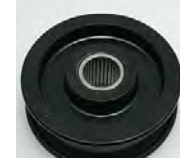
Idler Pulley, Flat Face, 4-3/8" OD, 1" Bore, 1-1/16" Face, 2-1/8" Shaft
