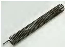
Spring, 1-1/4" OD X 1" ID X 9" Long, .1 End Closed, 1 End Straight out 90 Deg.
