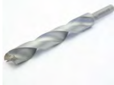
Twist Drill, 15/16" Dia., 6" Twist, Brad Point, Carbide Tipped, 1/2"
