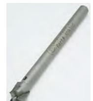
Router Bit 3-Wing, 3/4" Dia., Carbide Tipped, 1/2" Shank, 6" OAL
