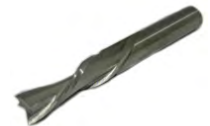
Router Bit, 3/8" Dia. X 3/8" Shank X 3" OAL, 1-1/4" Cutting Length, Double Edge Spiral Right Hand/ Down Cut, Solid Carbide
