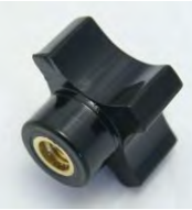
Knob, DK-83, 4-Prong (1-1/4 Dia.) 1/4-20 X 7/16 Deep Blind Hole Brass Insert.
