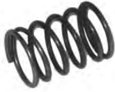
Spring 19/32"-ID X 1-1/16" Long, .062 Wire 6 Coils Ground Ends
