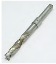
Twist Drill, 7/16" Dia., 3" Twist, Brad Point, 3/8" Modified Shank, 5" OAL.
