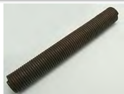
Spring, 1-3/4" OD X 1-1/4" ID X 12-3/4" Long, .207 Wire C/G, 59 Coils
