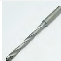
Twist Drill, 3/8" Dia. , 4" Twist, Brad Point, Carbide Tipped, 1/2" Shank,
