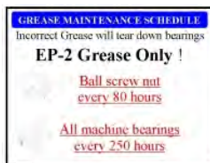
Label, Grease Maintenance Schedule, EP-2 Grease Only
