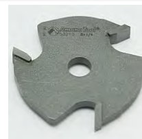
Router Bit, 3 Wing Slotting Cutter, 1/4 Kerf, 1-7/8" Dia., 5/16" Bore KVAL P/N: AMA53210
