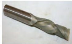
Router Bit, 5/8" Dia. X 5/8" Shank X 5" OAL, 2-1/4" Cutting Length, 2 Flute Spiral Chip breaker Compression Bit, Solid Carbide
