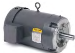
Motor, 3 HP, 3450 RPM, TEFC 145TC, 208-230/480 Volts (555)
