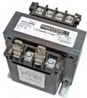
Transformer, 100VA, Primary Volt: 208/230/460V, Secondary: 120V, MI-
