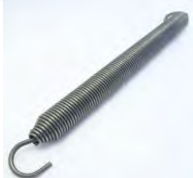
Spring, 1-1/2" OD X 19-3/8" Long .162 Wire. 4.03 LBS Per Inch 83.60 Load (SPC-10606) (990-FX Upper Spring)
