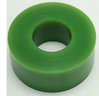
Roller Green Polytube, 3" O.D. X 1-3/8" I.D. X 1-1/4" Wide, 60 Duro
