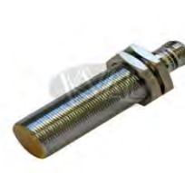
Sensor, 18mm Dia. Shielded Prox M12, Conn Turck BI5-M18E-AN6X-H1141, 56mm Threaded Barrel 71mm OAL.
