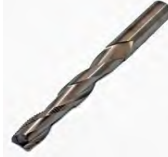
Router Bit, 1/2" Dia. X 1/2" Shank X 5" OAL, 2.7" Flute Up-Shear & Down-Shear, Compression Bit, ESG Coating, Solid Carbide
