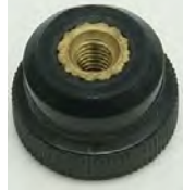
Knob, DK-41, Knurled, 3/4 Dia. 10-32 Female Insert 5/16 Thread Depth.
