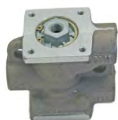
Valve, Humphrey, Air Piloted 501A-3-12-20, 1/2 Ports, 275 CFM AT 125 PSI 2&3WAY,N/0&C
