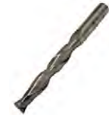
Router Bit, Solid Carbide, 3/4" Dia. X 3/4" Shank X 8" OAL X 2.2" CL Up Cut, 2 Flute Rougher With 5-1/2" Spiral Relief
