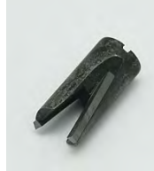
Router Bit, Spin On, 7/16" Dia., 1/4-28 Thread, Reverse Helix.
