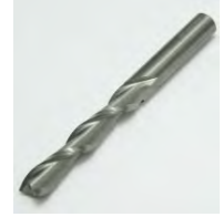
Router Bit, Solid Carbide, 1/2" Dia. X 1/2" Shank X 5" OAL X 2-3/4" CL 2 Flute Downcut, Left Hand
