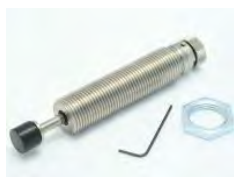
Shock Enidine OEM .50B 3/4-16 Thread 1/2 Stroke.
