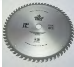
Saw Blade, 12" X 60 Tooth X 1" Bore (.118 Tooth Width)
