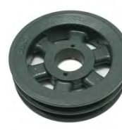
Gearbelt Pulley, 2BK67H, Double Sheave 6.45" OD. Use H Bushing
