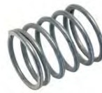
Spring 19/32-ID X 7/8 Long, .062 Wire 5 Coils Ground Ends
