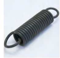
Spring, 1-1/8-OD X 3/4-ID X 4-3/4 Long with Hooked Ends
