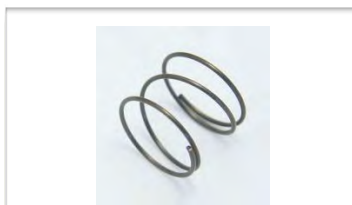
Chuck Spring-.032 Music Wire 5/8-Dia 5/8-Long Closed Ends.
