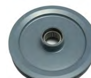
Pulley, BROBK65, Modified Bore to 1.313 +.000/-0.001 For BH1612 Needle Bearing
