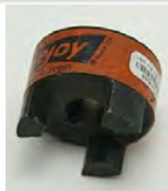
LoveJoy, L075 Coupling Body, 5/8" Bore, Part of 3 Piece Flexible Coupling With 3/32" Keyway and (2) 1/4-20 Set screws
