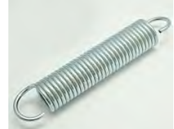
Spring, 1-1/4" OD X 7/8" ID X 7-1/4" Long, .162 Wire Hooked End
