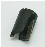
Router Bit, Spin On, 5/8" +.005" Dia., 1/4-28 Thread, Reverse Helix.
