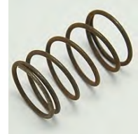
Spring, 1-1/4" OD X 2" Long, .090 Wire Coarse Ground
