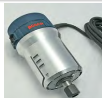
Router, Bosch, Motor Only, 2 HP, 120 VAC, 11 amp, 25,000 RPM, 1/2 Collet
