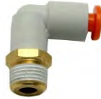
Fittings, Male Swivel Elbow KQ2L Series, 1/4 Tube OD X 1/8" NPT
