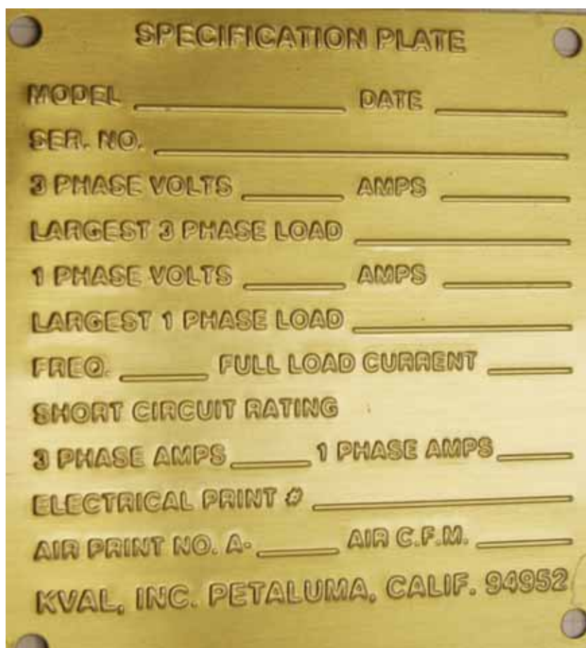
FIGURE 1-1. Example of KVAL Specification Plate
